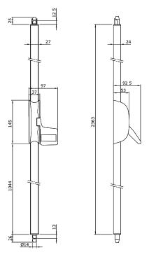
Emergency exit device "Pad Bolt" operated by means of PUSHING PLATE FOR FIRE RESISTANT DOORS,
