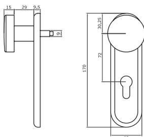
**Plate with knob and cylinder hole.**
