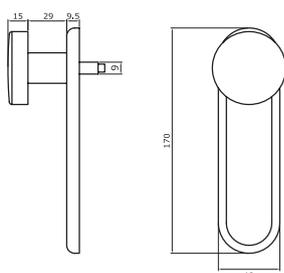
**Plate with knob and without cylinder hole.**
