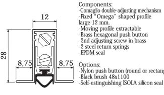
Components: -Comaglio double-adjusting mechanism -Fixed "Omega" shaped profile large 12 mm. -Moving profile extractable -Brass hexagonal push button -2nd adjusting screw in brass -2 steel return springs Options: -Nylon push button (round or rectangular) -Black brush 48x1100
