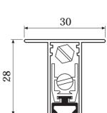
Components: -Comaglio double-adjusting mechanism -Fixed "T" shaped profile -Moving profile extractable -Brass hexagonal push button -2nd adjusting screw in brass -2 steel return springs -EPDM seal
