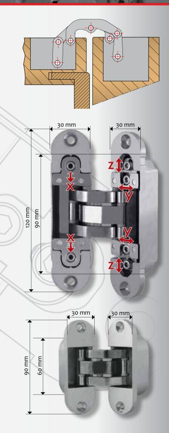
Available in white zinc finishing. Other finishes also available on request. Capacity - adjustable version : 50 kg. Capacity - non-adjustable version : 35 kg. Door opening angle : 180°.
